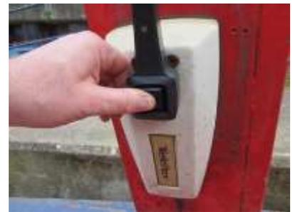
Once this has been done, turn the key one step further to the START position. The engine should turn and fire up. Release the key and it will turn back to the ON position.
