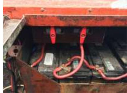
Once the battery isolator switch is turned on, the engine compartment bilge pump may start – this boat is fitted with an automatic bilge pump with manual over-ride, so this is normal behaviour.
